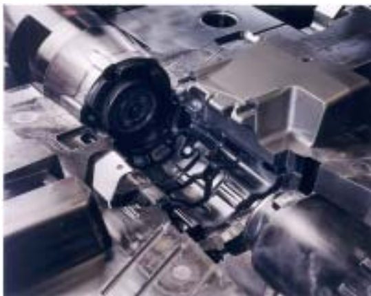
Die for hydraulic top slide
